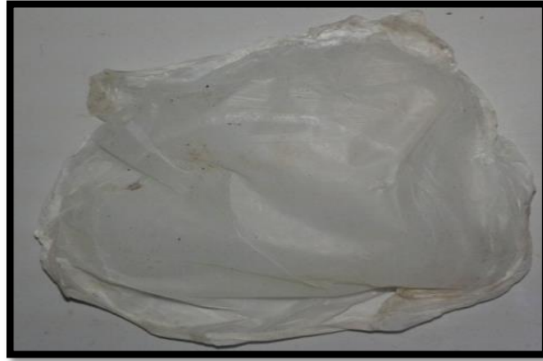
Figure(1): air filter membrane after air filtration.
