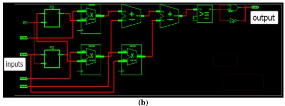
$Fig. 5\ (a\ )\ Time\ diagram,\ (b) Hardware\ circuit\ , of\ implementing\ an\ \ 8-bit\ neuron\ with\ hardlims\ activation\ function\ .$
