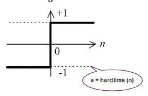
Fig.(4) Symmetrical hard limit activation function
