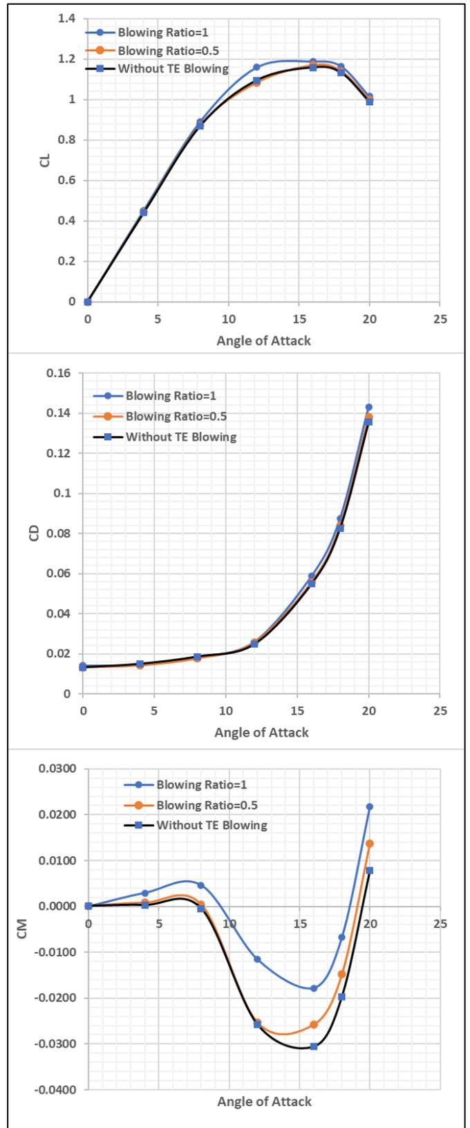
Fig. 9 NACA0018 aerodynamic performance at different blowing ratio at Reynolds number  $13.7 \times 10^5$ .
