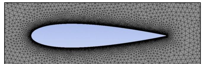
Fig. 3 Mesh intensity at the airfoil Wall.
