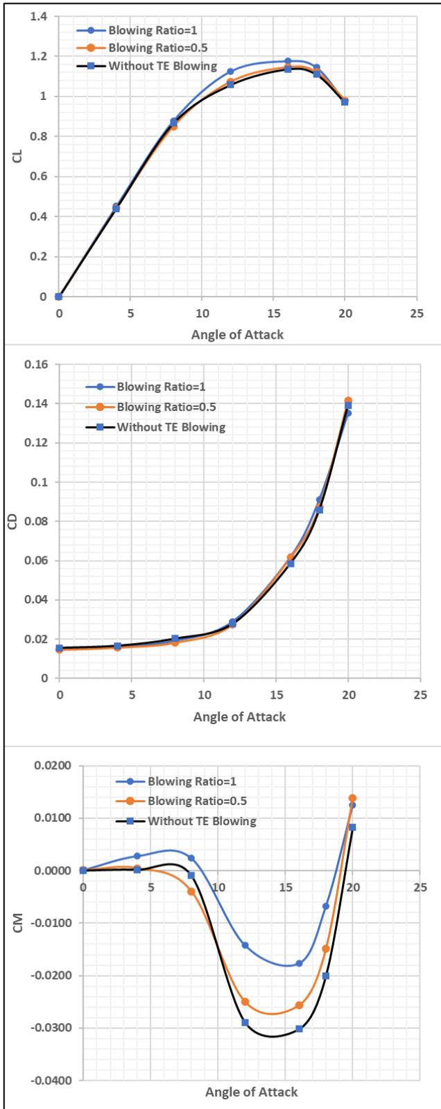
Fig. 6 NACA0018 aerodynamic performance at different blowing ratio at Reynolds number  $6.85 \times 10^5$ .
