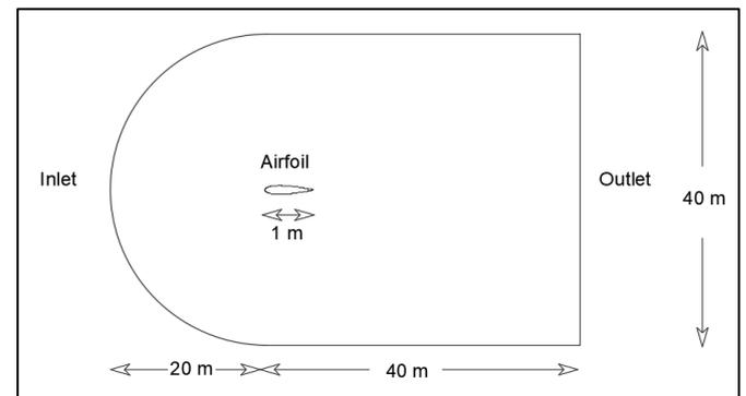
Fig. 2 schematic drawing for the flow domain and its boundary condition.
