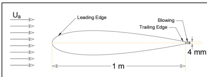
Fig. 1 NACA0018 airfoil geometry with blowing jet at the trailing edge.
