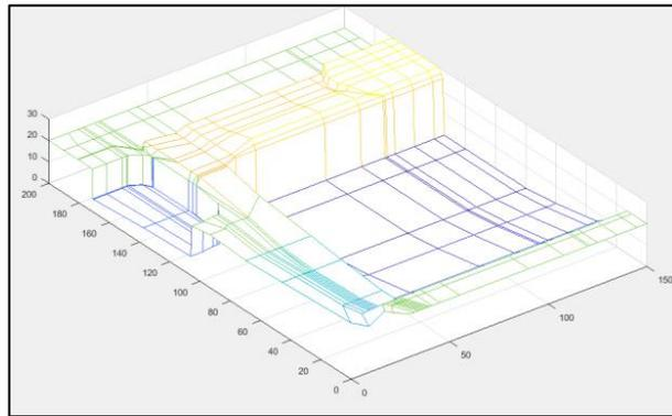
**Figure 8: The mesh of control points of backdoor design**
