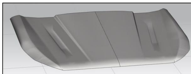
**Figure 7: true shading of the car hood surface (NX).**
