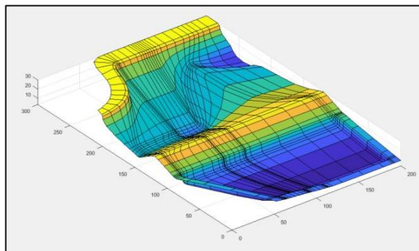
**Figure 3: the designed surface of car exterior door (MATLAB).**
