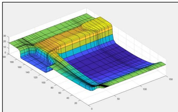
**Figure 9: the designed surface of back car door design (half)**
