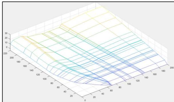
**Figure 5: the control point mesh of car hood design**
