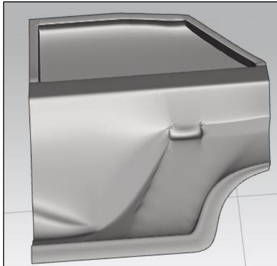
**Figure 4: true shading of the designed surface (NX)**
