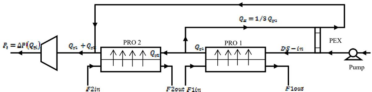
Fig. 2: first enhancement PRO process cycle
