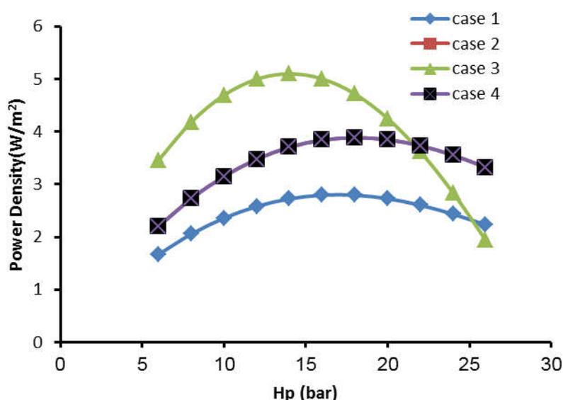
Fig. (6): Power density versus the hydraulic pressure
