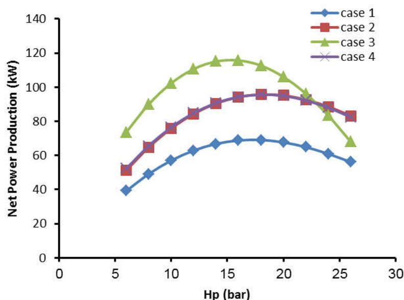
Fig. (7): Net power production versus the hydraulic pressure supplied
