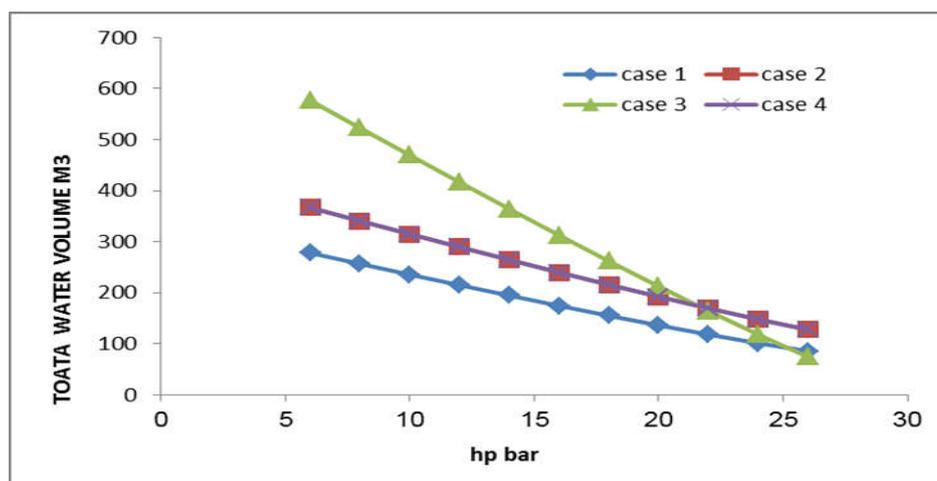
Fig. (5): Total volume of water produced versus the hydraulic pressure supplied
