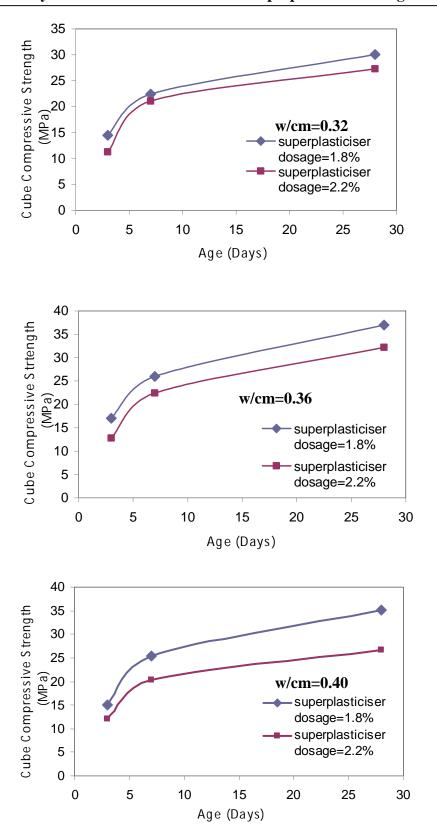
Fig.(6)The Relation between Cube Compressive Strength and Age of Curing
