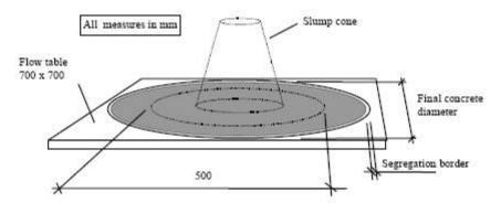
Fig. (1) The Slump Flow Test
