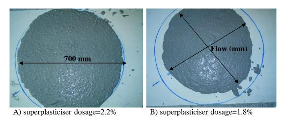
Fig.(3) The Flow of Mix in Slump-Flow Test
