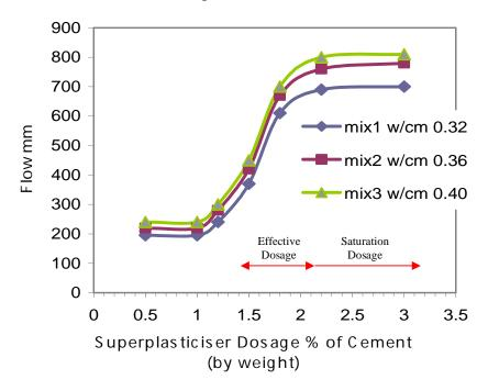
Fig.(2) The Relation between Flow and Superplasticiser Dosages
