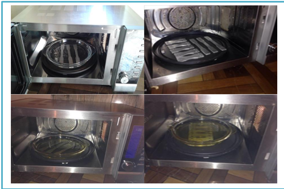
Figure (1): Microwave Furnace with Specimen
