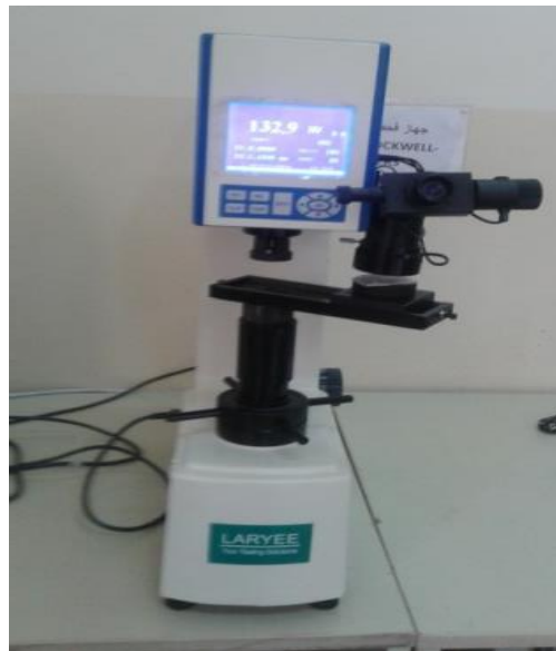
Figure (4): Rockwell Hardness Testing Machine
