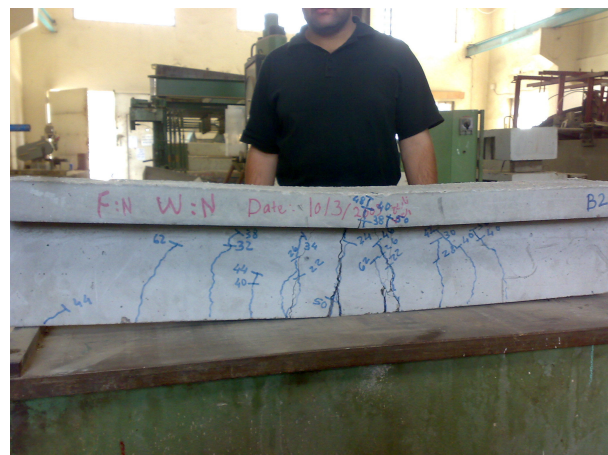
Fig.3 Cracks pattern of beam B2
