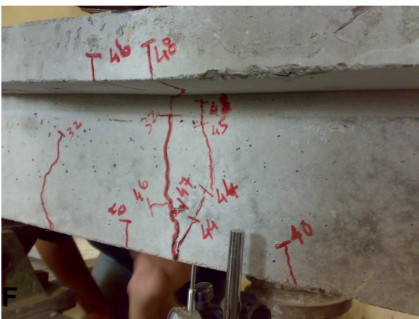
Fig.2 Cracks pattern of beam B1
