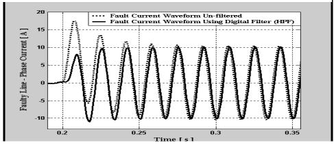
Fig. (9):- Current waveforms of fault using dc - offset removal filter at fault inception =  $0^{\circ}$  and fault location =  $50^{\circ}$
