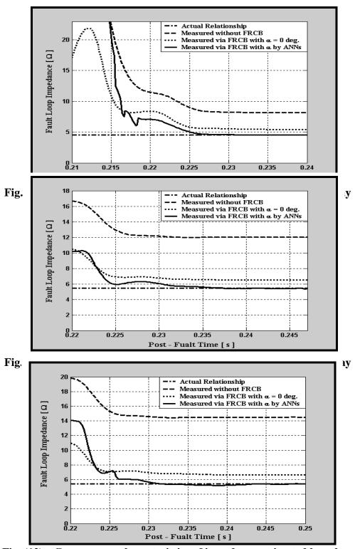
Fig. (12):- Convergence characteristics of impedance estimated by relay at fault location = 50% and  $R_{\rm F}$  =20  $\Omega$  using (FC-DFT)
