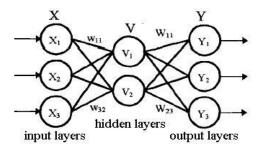
Fig. (3):- Three-layer Neural Network Architecture
