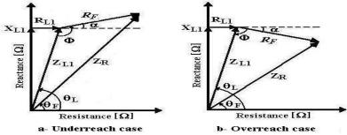
Fig (6):- Apparent impdance deviation with significant fault resistance
