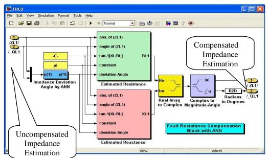
The I Fig (7): - Simulation of a Fault Resistance Compensation Block [FRCB] with ANN using *Matlab/Simulink* of the PSB
