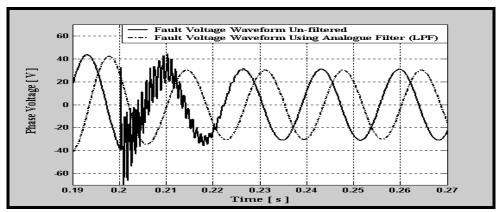
Fig. (8):- Voltage waveforms of fault using anti - aliasing filter at fault inception =  $-90^{\circ}$  and fault location =  $50^{\circ}$
