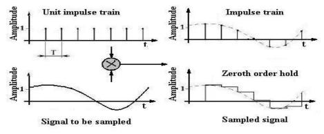
Fig. (5):- The comparison of sampling between Unit impulse train Digital Filter (Mimic Filter) and Zero order hold
