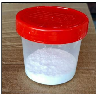
Fig. 3 Alumina nanoparticles prepared by Sol-Gel process.
