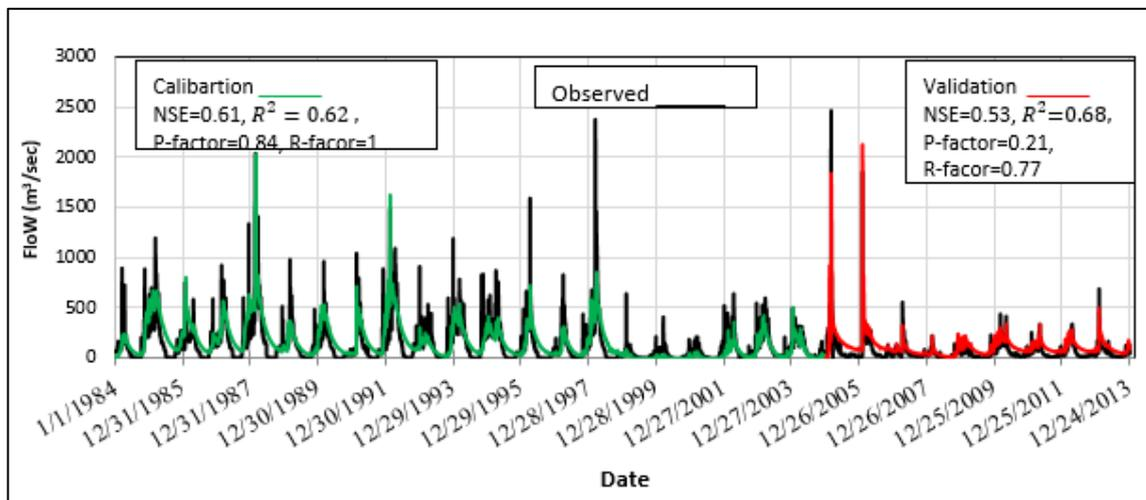
Figure 6: The calibrated and validated stream flow
