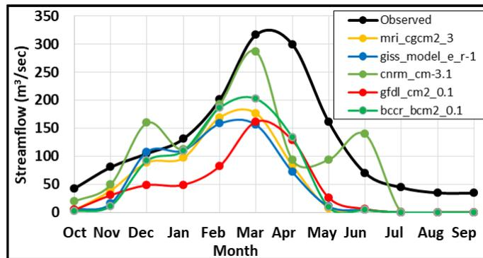
Figure11: Potential stream flow under climate change condition until 2050
