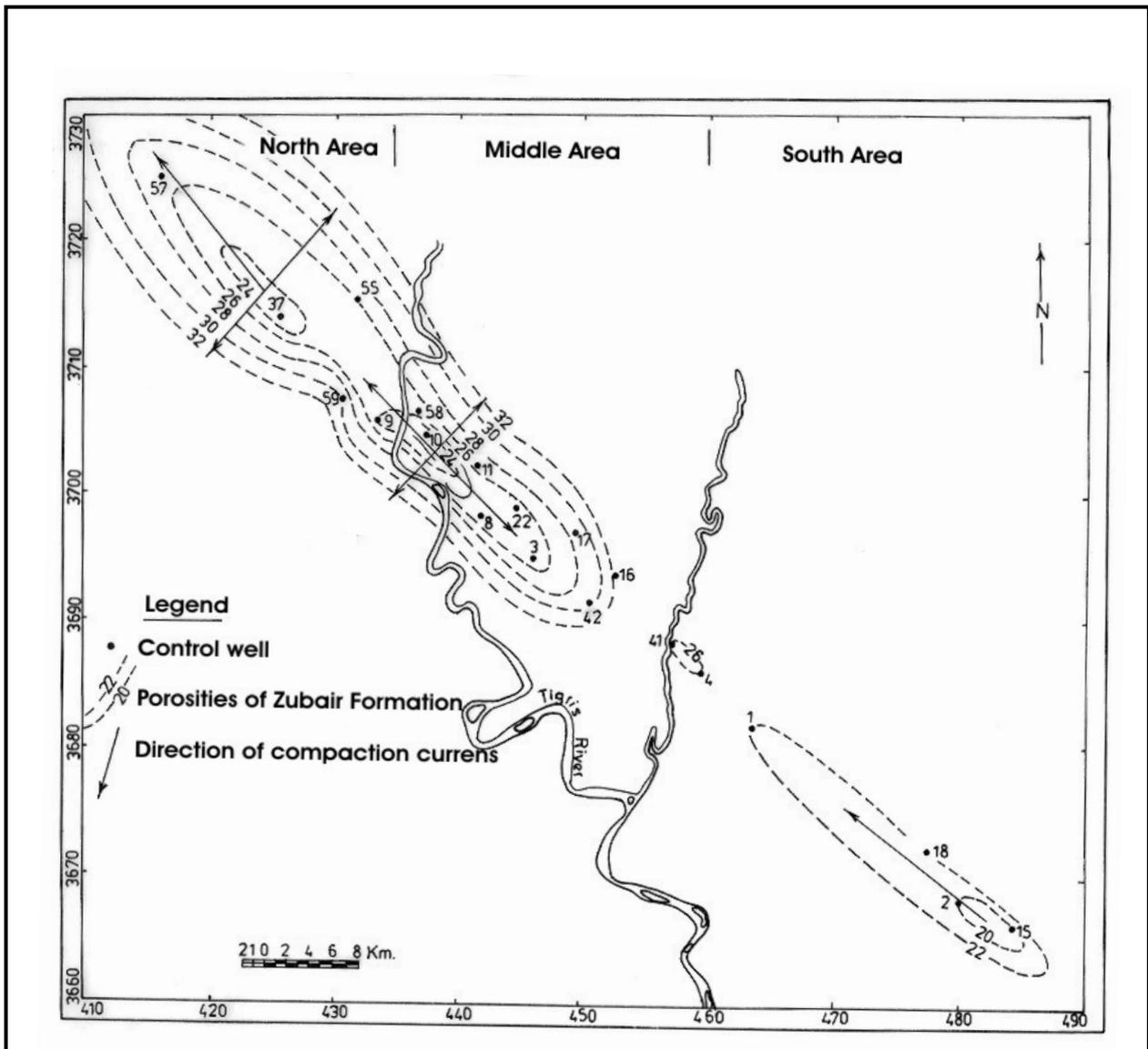
Fig. 10 : The varied direction of compaction current in the mudstone of Zubair formation.
