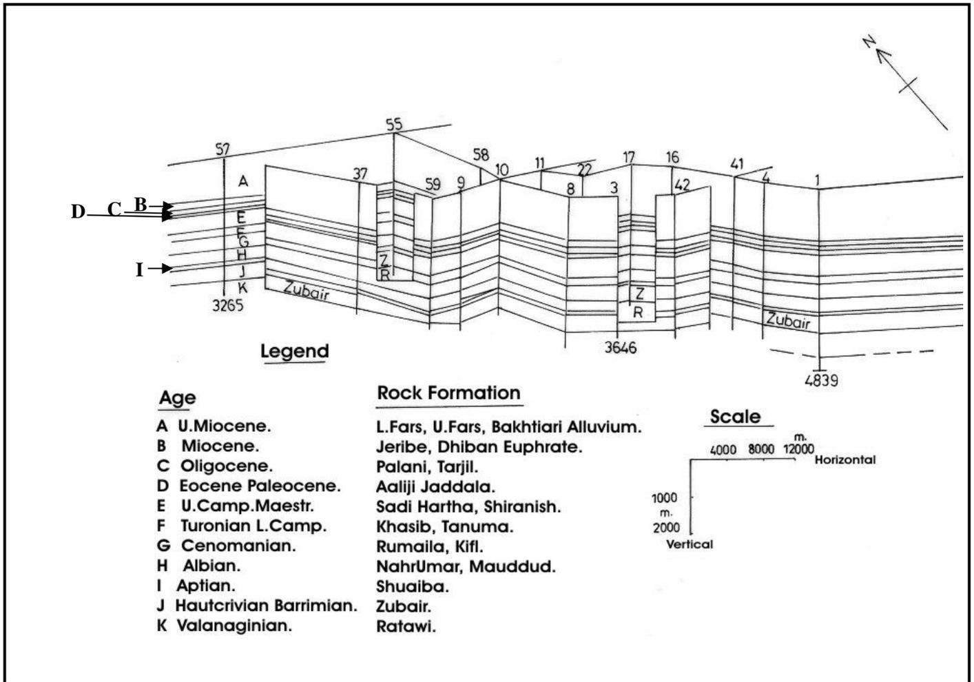
Fig. 4 : Panel diagram of East-Baghdad oilfield.
