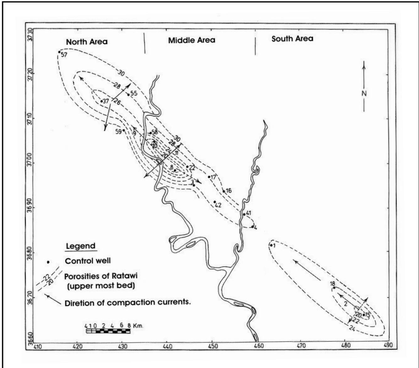
Fig. 9 : The varied direction of compaction current in the mudstone of Upper Ratawi
