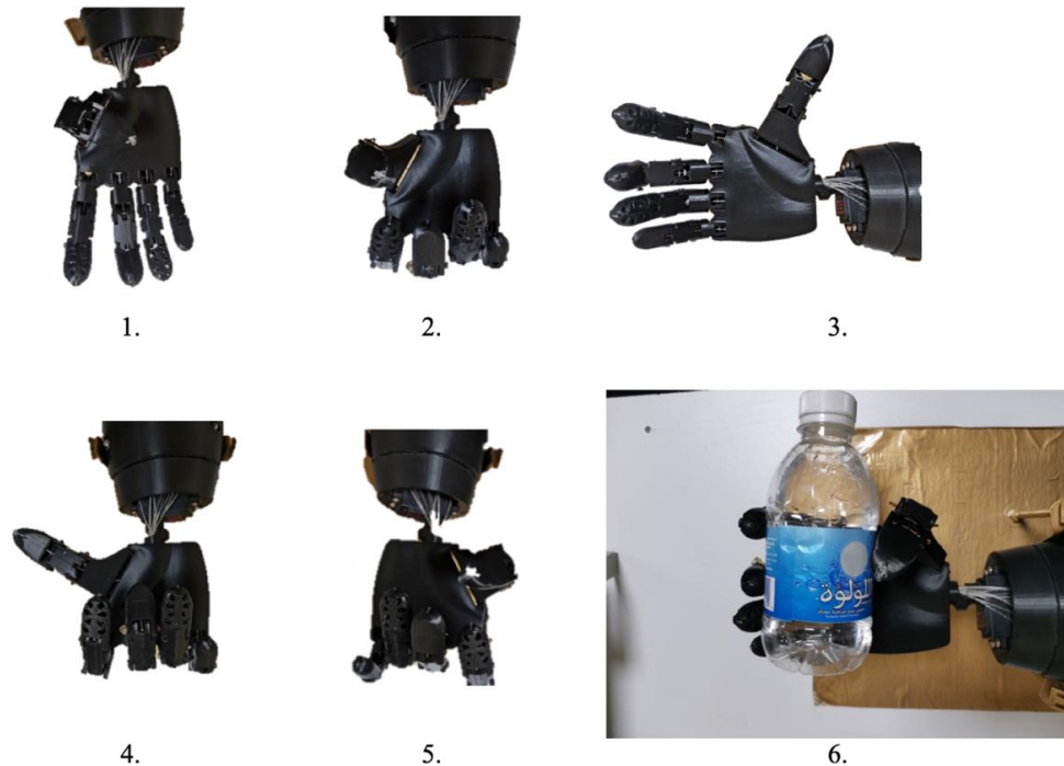
Fig. 7 The prosthetic hand movements: (1) Hand shake, (2) Fingers closed, (3) Fingers open, (4) OK gesture, (5) Half open, and (6) Grabbing an object.
