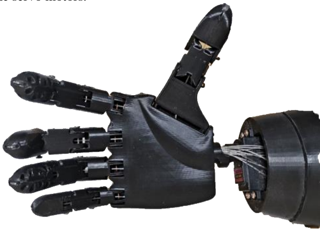
Fig. 5 The 3D printed prosthetic hand.
