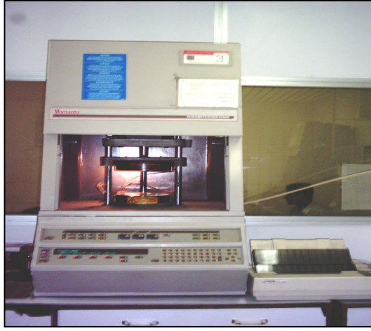
الشكل (1) : جهاز (Oscillating Disk Rheometer)
