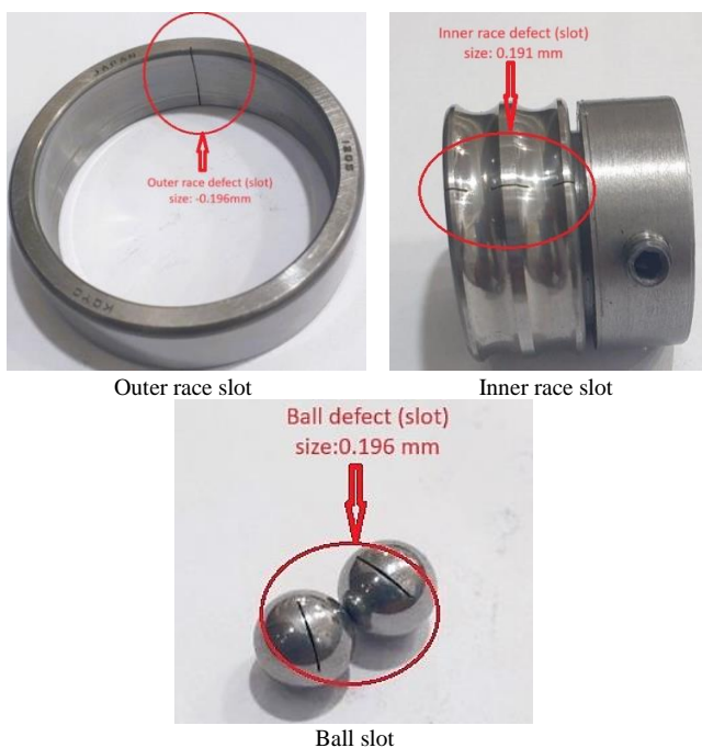
Fig. 8 Types of defects in the used ball bearing.
