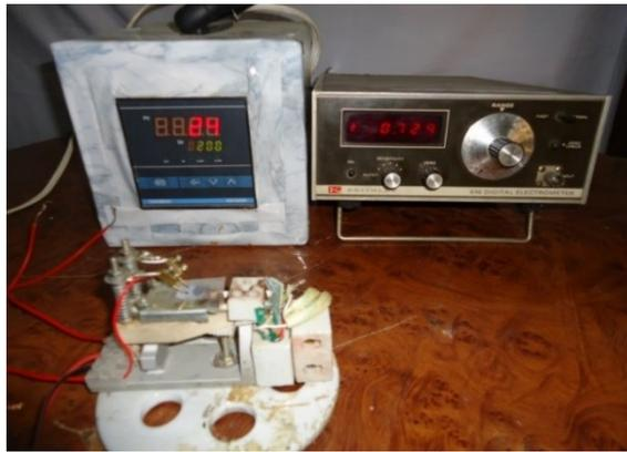
Figure 8: Photograph represents a home-made thermal and electrical measurement stage.
