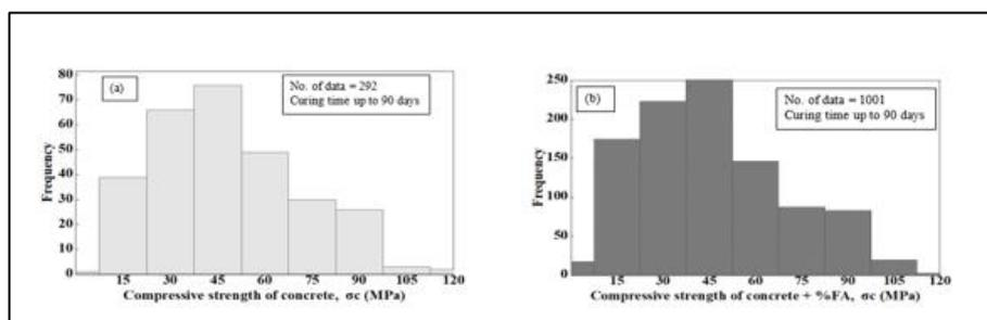
Figure 3: Histogram of compressive strength ( $f_c'$ ) of (a1) concrete and (b) concrete modified with FA
