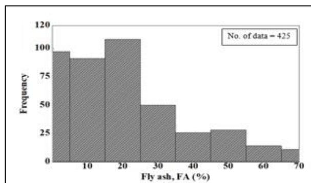
Figure 2: Histogram of percent of fly ash, FA (%) added to the concrete
