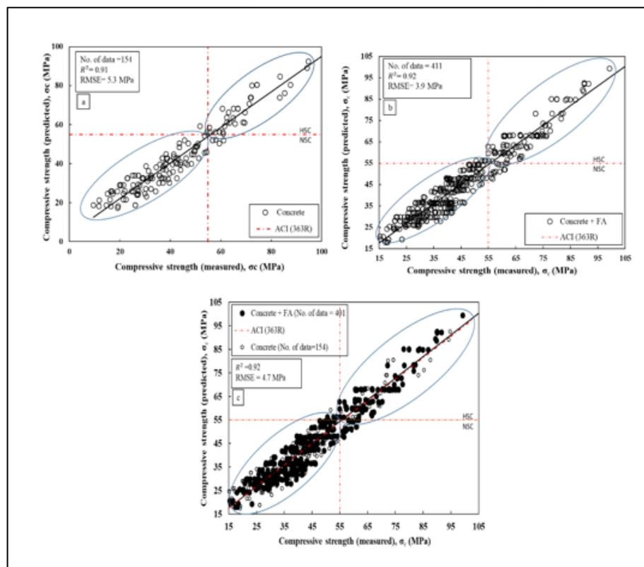
Figure 6: Relationship of predicted and measured the compressive strength ( $f_c'$ ) of NSC) and HSC (a) concrete (b) concrete modified with FA and (c) concrete + concrete modified with FA
