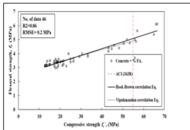
Figure 9: Relationship between flexural and compressive strength of concrete modified with fly ash
