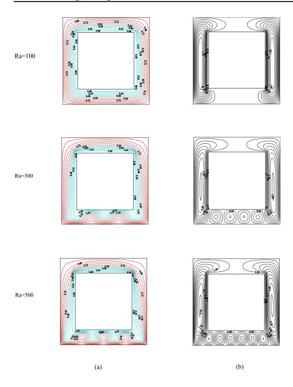
Figure ( 5 ) (a ) Isotherms, ( b ) Streamlines at body size ( 2/3x2/3 )and different rayleigh number
