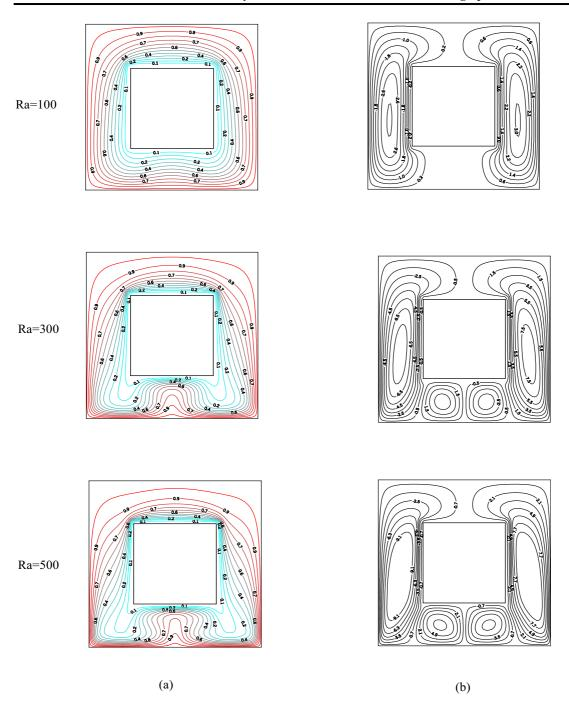
Figure (4) (a) Isotherms, (b) Streamlines at body size (1/2x1/2) and different rayleigh number
