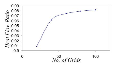
Figure(2) Relation Between Heat Flow Ratio and no. of Grids for Body Size 1/2x1/2 and Ra=200
