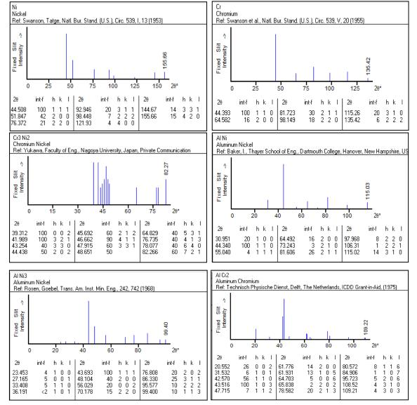
Fig. (3) Standard XRD for main intermetallic phases according to JCPDS cards.
