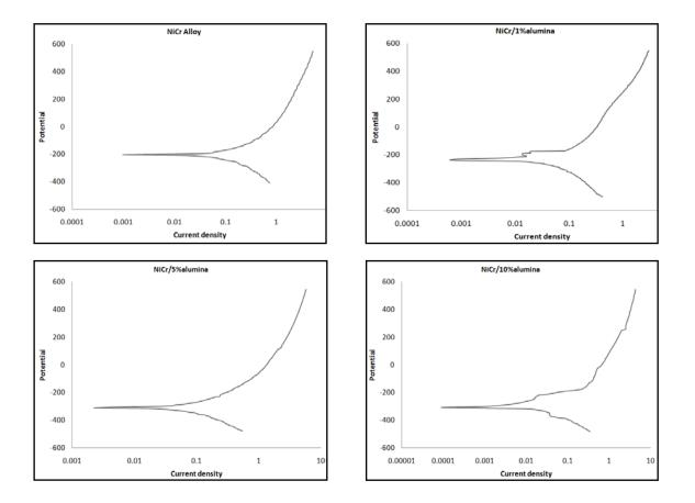
Fig. (5) Tafel plots of Ni-Cr alloy and its composites in saliva at 37°C.
