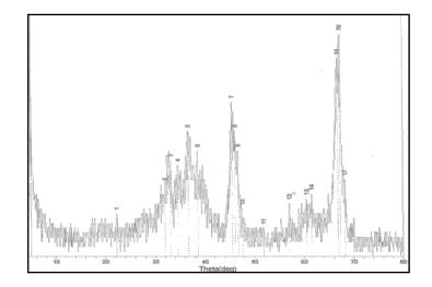
Fig. (1) XRD of alumina.
