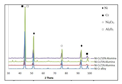
Fig. (2) XRD patterns for Ni-Cr alloy and its composites.
