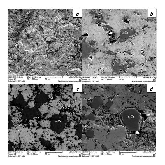
Fig. (4) SEM images of Ni-Cr alloy (a) and its composites reinforced by 1%Alumina (b), 5%Alumina (c) and 10%Alumina (d).
