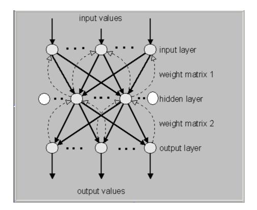
Figure 1. The network topology used in BP algorithm.
