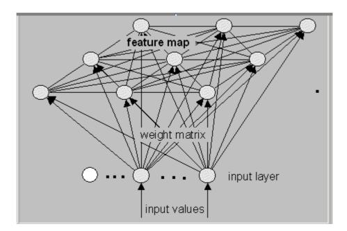
Figure 2. The network topology used in SOFM algorithm.
