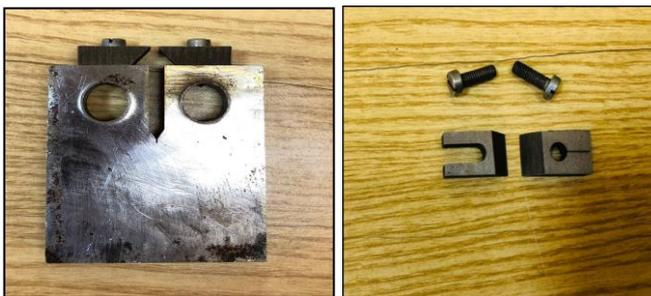
Fig.16 Attachable knife-edge design.
