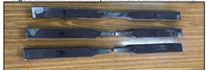
Fig.4 Tensile test specimens after a fracture.
