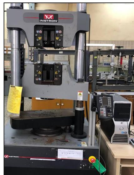
Fig.5 INSTRON Tensile Test Machine.
