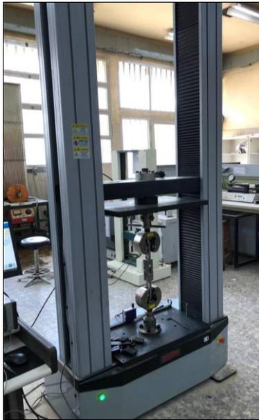
Fig.19 100kN Universal Testing Machine.
