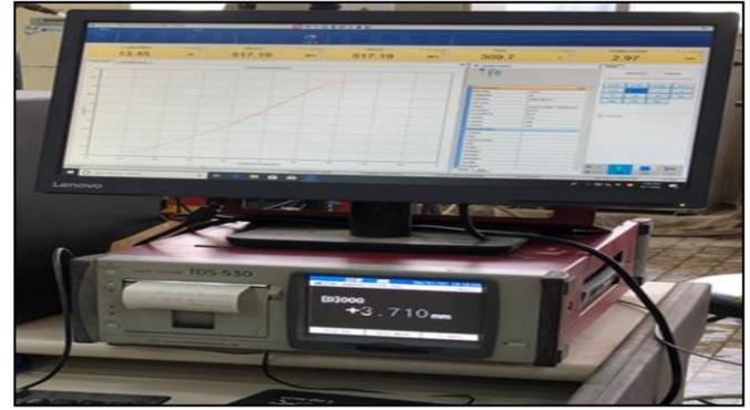
Fig.22 PC and displacement transducer.
