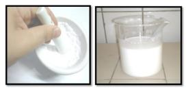
Figure 2: Modified nanoparticles before and after dryness A: silanol containing nanoparticles; B: nanoparticles after 14 days.
