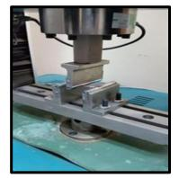
Figure 6: Instron (examination machine for flexing test)
