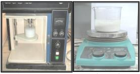
Figure 1: equipment used for surface modification of nanofillers A: probe sonication apparatus; B: magnetic stirrer.
