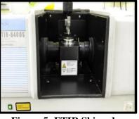
**Figure 5: FTIR Shimadzu** spectrophotometer.
