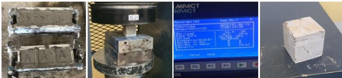
**Fig. 1. Casting and testing of cement mortar cubic sample****Table 4. Test results of mortar cubic samples**
