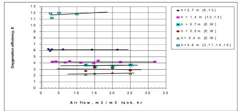
Fig (4): Effect of air flowrate (D) on the oxygenation efficiency of the system at different (h) values. E.W:
