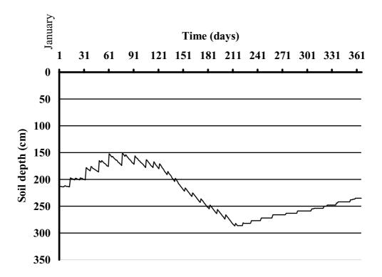
Figure(2)Water table hydrograph for the collector zones in the Dujailah project.
