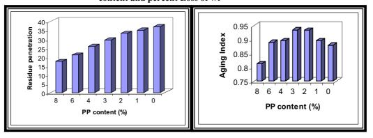
Fig. (5) Relationship between Polypropylene<br/>content and Residual PenetrationFig. (6) Relationship between Polypropylene<br/>content and Aging Index
