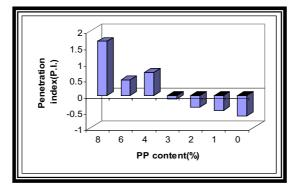
Fig. (1) Relationship between Polypropylene content and Penetration
