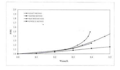
Fig (3): relationship of  $(P/P_{E})$  verses  $(w_{max}/L)$  for fixed ended column.
