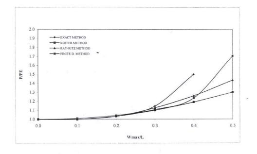
Fig (2): relationship of (P/P<sub>E</sub>) verses ( $w_{max}/L$ ) for pin ended column.
