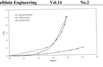
Fig (1): Comparison of  $(P/P_E)$  verses  $(w_{\text{max}}\!/\!L)$  for different columns.
