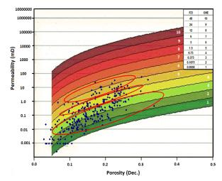
Fig. 4. Porosity- Permeability Data Drawn on Standard GHE Plot
