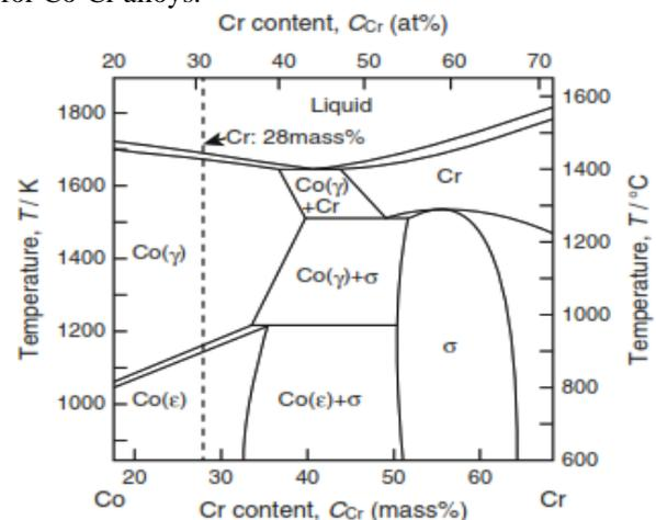
Fig.1 Equilibrium phase diagram of Co-Cr alloys [9]
