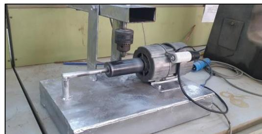
Fig. 4 Pin on Ring device of Wear Testing
