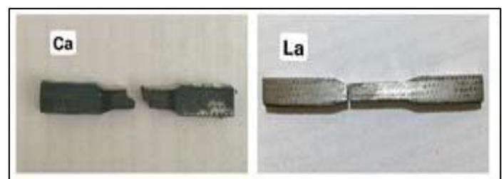
Fig.3 Two types of Tensile samples after Testing
