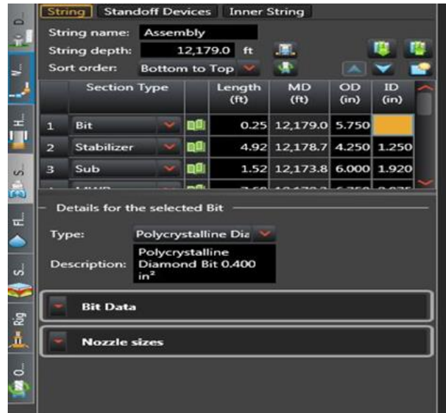
Fig. 6. Drill string components for ZB-250
