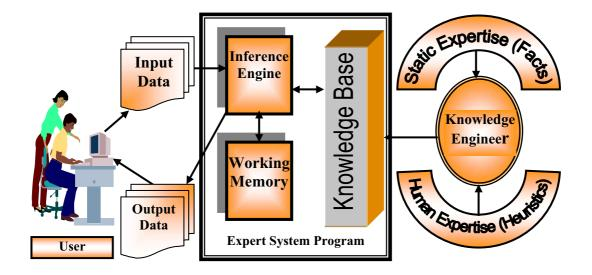
Figure (1) Expert System Architecture.
