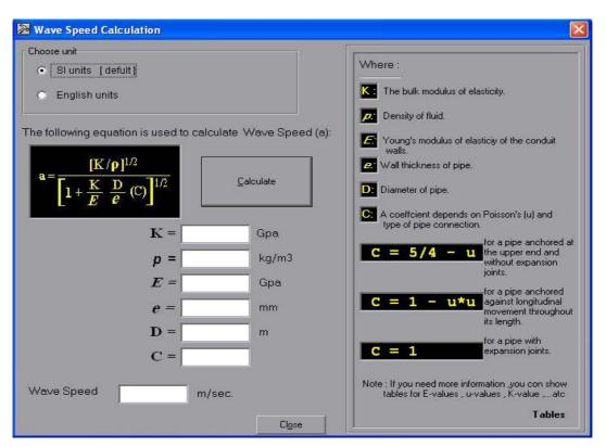
Figure (7) Window Used to Calculate Wave Speed.
