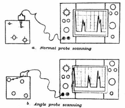
Fig.(2) (a,b) Typical normal and angle wave probe scanning at 1/2 skip for maximum echo height from side drilled hole, showing construction and mode of operation
