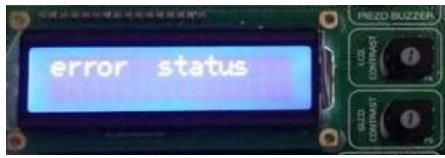
Figure 18 . Error status appears on LCD when fault occurs
