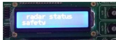
Figure 17. {a, b, c} Shows LCD display for (short, middle, large) range region respectively with EasyPIC v7 board.
