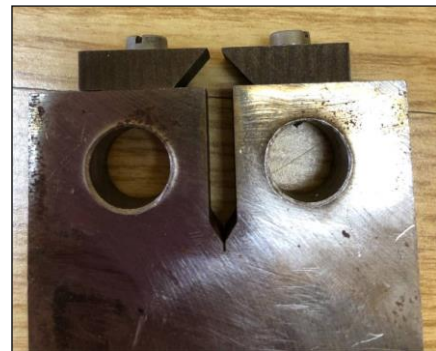
Fig. 8 Pre-cracking by WEDM.
