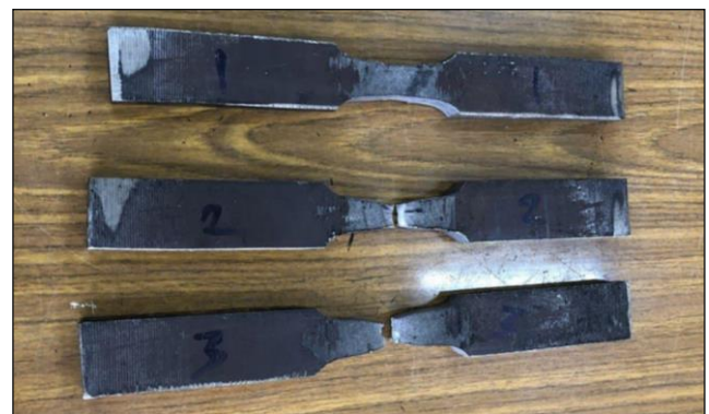
Fig. 5 Tensile test specimens after a fracture.
