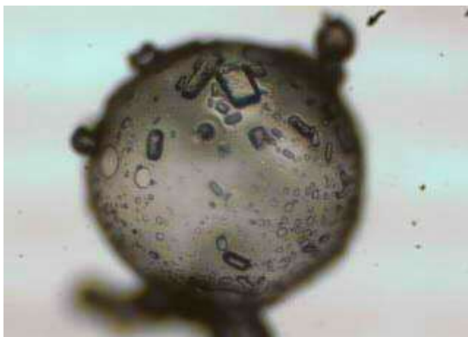
Figure-4: CA microspheres (FC1) as seen by optical microscopy under (10x SF)
