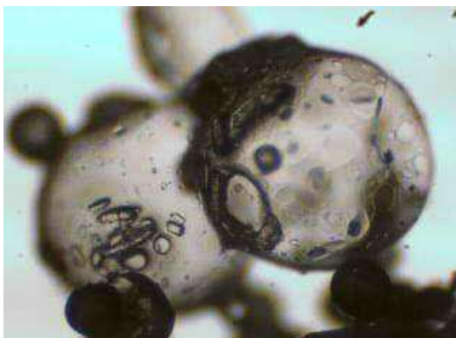
Figure-3: CA microspheres (FC1) as seen by optical microscopy under (10x SF)
