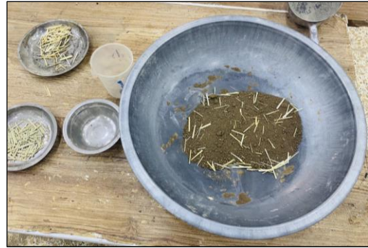
Fig. 3 Mixture of randomly distributed fibers and moist soil.
