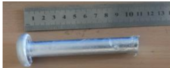
Fig. 2. Sample after the casting process
