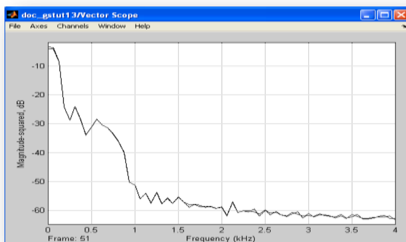
Fig (5) Viewing Spectrogram of the Speech Signal using MATLAB Signal Processing Block set
