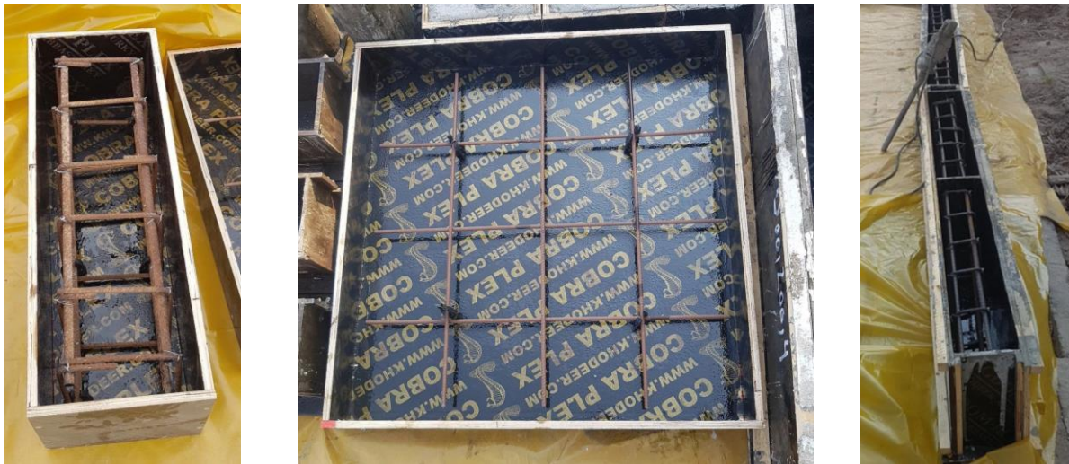
Fig. 3 Forms and Reinforcement of the Specimens.
