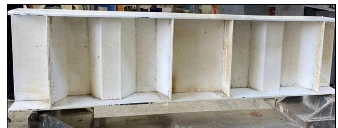
Fig. 11 Beam with trapezoidal corrugate and thickness 1 mm (B6).
