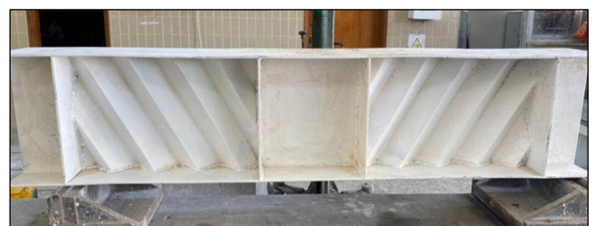
Fig. 12 Beam with inclined corrugate web and thickness 1 mm.
