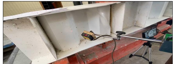
Fig. 37 Trapezoidal corrugated beam with thickness 1 mm B6.
