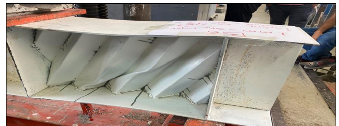
Fig. 38 Diagonal corrugated beam with thickness 1 mm (B7).
