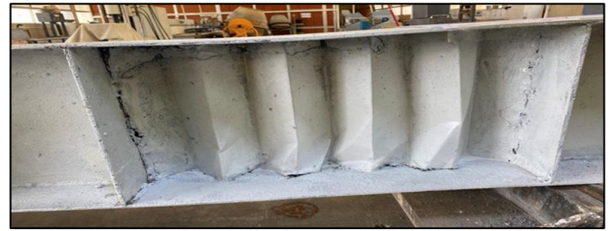
Fig. 35 Corrugated beam with one layer and thickness 0.5 mm B4.
