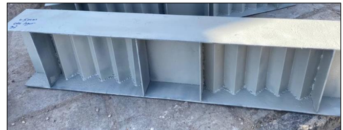
Fig. 9 Beam with corrugate web one layer and thickness 0.5 mm (B4).
