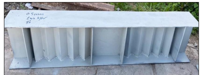
Fig. 10 beam with corrugate web two layer and thickness 0.5 mm (B5).
