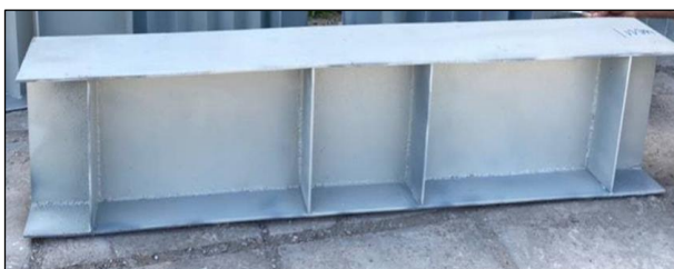
Fig. 6 Control model without corrugate web (B1).
