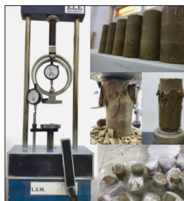
Fig. 1 Preparation and testing of UCS samples with additives.
