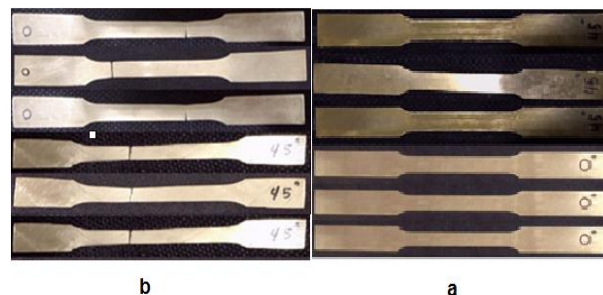
Figure 3: Tensile specimens (a) before test (b) after test
