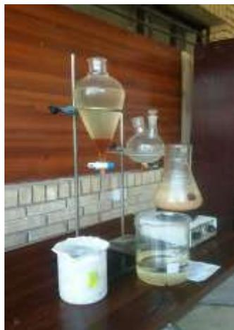
Figure 2: The biodiesel preparation system
