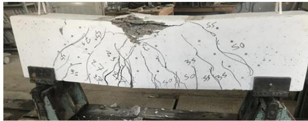
**Plate 4: Cracks pattern of beam B3**
