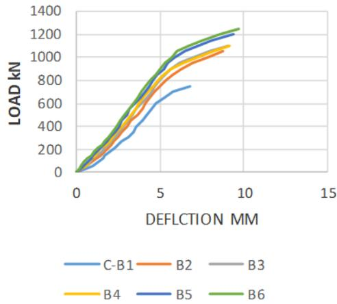
Figure 4: (Load-deflection)-curves of deep beams specimens
