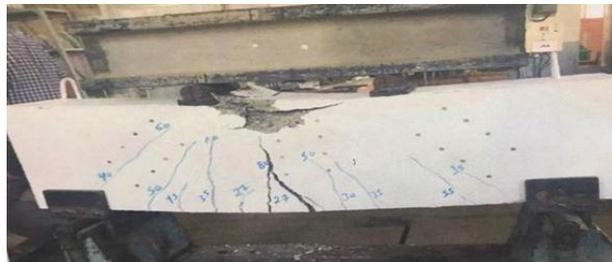
**Plate 5: Cracks pattern of beam B4**
