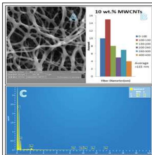
Figure 6: PVA /10 wt% MWCNT electrospun film (A) electron microscopy picture, (B) fibers dia. histogram, and (C) chemical component.
