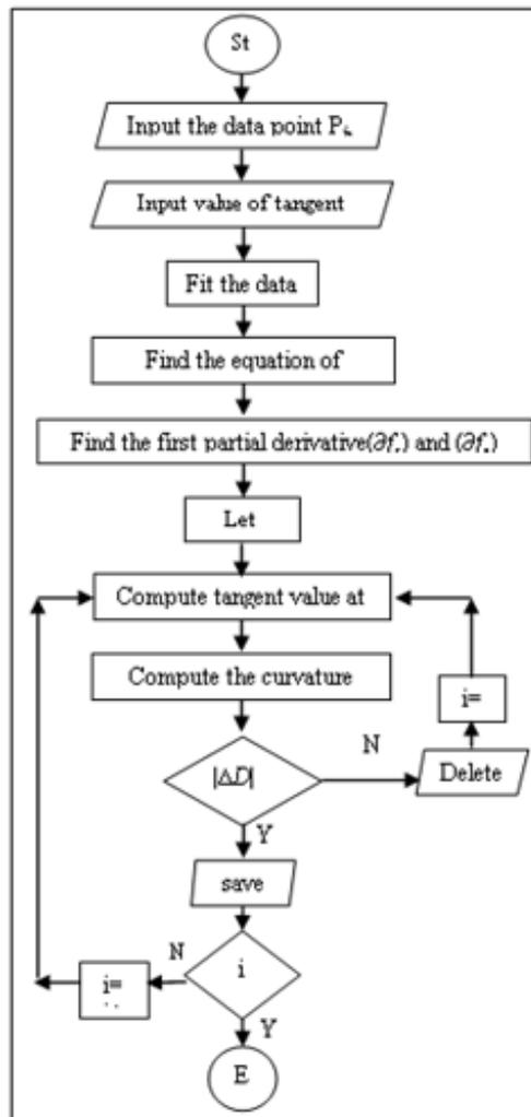
Figure 3: Flow chart of Tangent Pre-Processing algorithm
