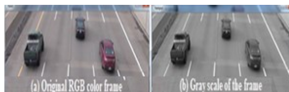
Figure 5: Conversion of an RGB frame to a gray scale frame
