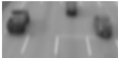
Figure 7: The distortion caused by large filter sizes
