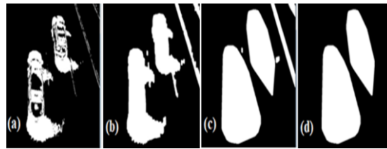
Figure 9: Effect of ignoring shadow problem (Moving objects extraction steps: a: thresholding b: applying contour c: applying convex hull d: image blob)
