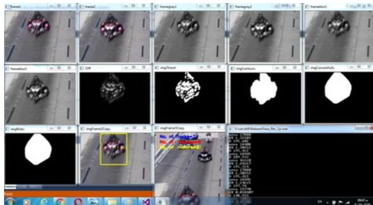
Figure 13: Steps of motorcycles detection and recognition
