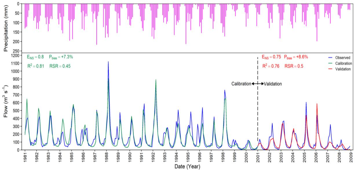
Figure 6: Monthly observed and simulated runoff at the Derbendi-Khan dam reservoir from 1981 to 2008
