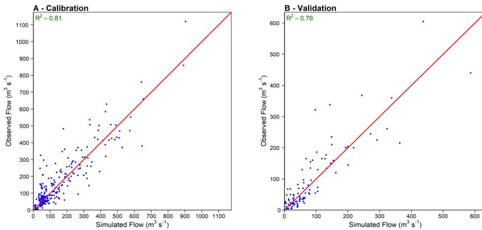
Figure 7: Correlation between monthly observed and simulated stream flow during calibration and validation periods
