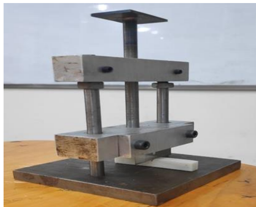
Picture 1. Method of creating incision for SENB fracture toughness samples
