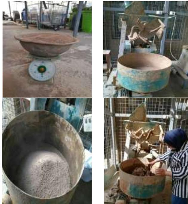
**Figure 2: Preparation of Clayey Soil by Grinding**
