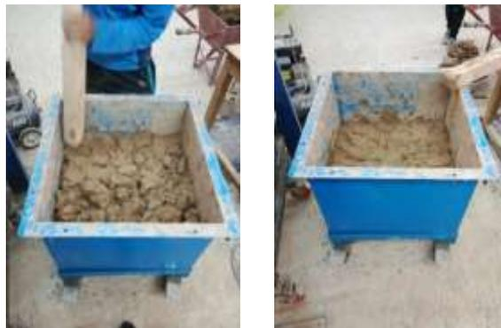
**Figure 3: Placing the Clay in the Box and Compaction Gently by Wooden Tamper to Avoid the Entrapped Air**
