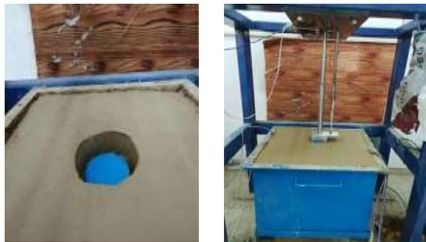
**Figurer 7: Footing at Surface and at Depth 5 cm.**
