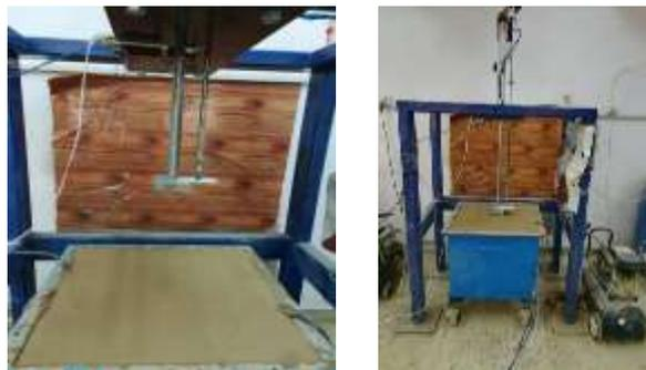
**Figure 4: Surface Adjustment of the Model and Carrying the Model into the Load Setup.**
