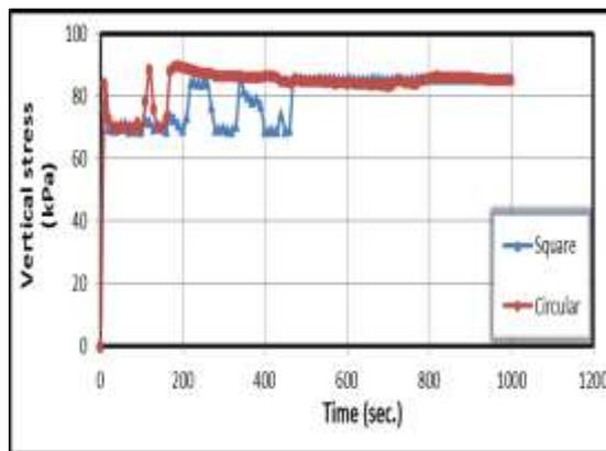
Figure 22: Vertical Stress Change with Time when  $c_u = 70$  kPa,  $D_f = 5$  cm, Velocity = 6 mm/sec at Depth 10 cm
