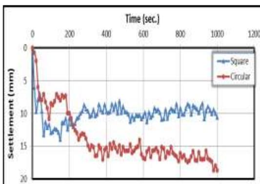
Figurer 12: Settlement Change with Time when the  $D_f = 5$  cm,  $c_u = 70$  kPa and Velocity = 6 mm/sec.
