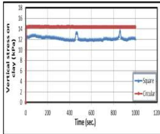
Figure 13: Vertical Stress Change with Time when  $c_u = 20$  kPa,  $D_f = 0$  cm, Velocity = 6 mm/sec at Depth 10 cm
