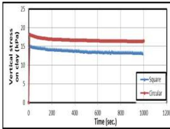
Figure 16: Vertical Stress Change with Time when  $c_u = 40$  kPa,  $D_f = 0$  cm, Velocity = 6 mm/sec at Depth 10 cm.
