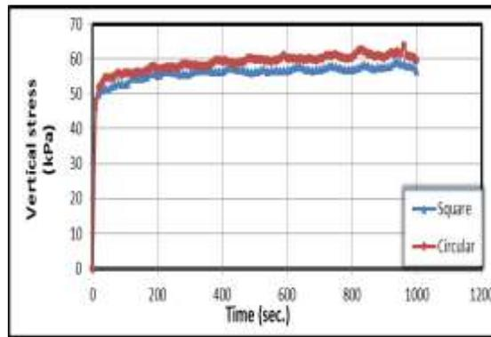
Figure 23: Vertical Stress Change with Time when  $c_u = 70$  kPa,  $D_f = \text{cm}$ , Velocity = 6 mm/sec at Depth 20 cm
