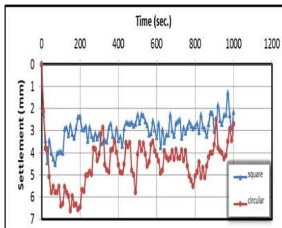
**Figure 8: Settlement Change with Time when the  $D_f = 0$ ,  $c_u = 20$  kPa and Velocity = 6 mm/sec**
