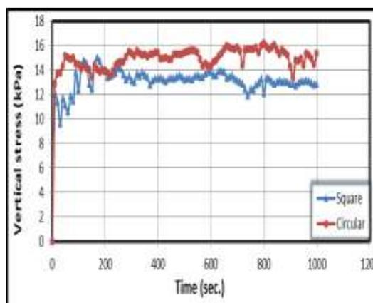
Figure 15: Vertical Stress Change with Time when  $c_u = 20$  kPa,  $D_f = 5$  cm, Velocity = 3 mm/sec at Depth 10 cm
