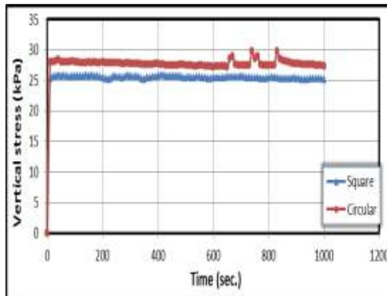
Figure 18: Vertical Stress Change with Time when  $c_u = 40$  kPa,  $D_f = 5$  cm, Velocity = 6 mm/sec at Depth 10 cm
