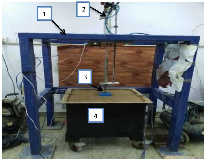
**Figure 1: Overall outlook of the produced device: 1. Steel load framing, 2. Axial load system, 3. Model footings, 4. Steeling box (test container)**
