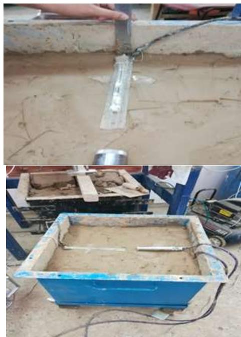
**Figurer 6: Installing Pressure Cells and Piezometer and Checking the Distance from Surface to Sensors Equal to  $B=10$  cm**
