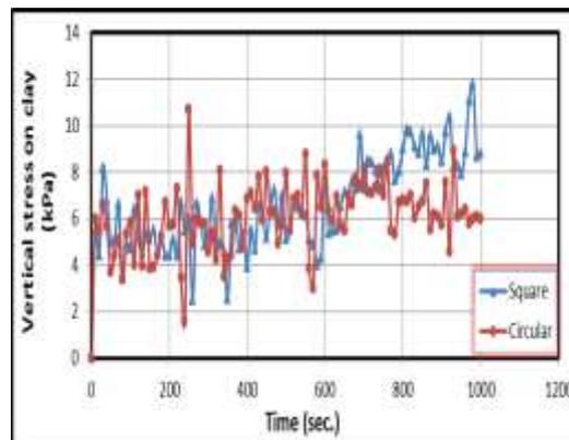
Figure 14: Vertical Stress Change with Time when  $c_u = 20$  kPa,  $D_f = 0$  cm, Velocity = 6 mm/sec at Depth 20 cm.
